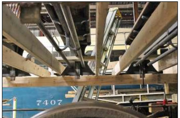
FROM LEFT SIDE TO RIGHT SIDE: This view shows Keith Bray's intricate support system was built to hold up the car's sides and roof.
