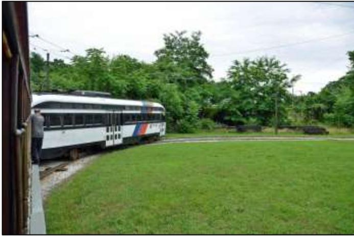
28<sup>TH</sup> STREET LOOP: Justin is watching #1164 from the front door of #26 as it rounds the curves to be sure #1164 did not derail. Ed watches from the front of #1164 while Mark kept a steady hand on the car's controller and brake. #1164 performed like a champ.
